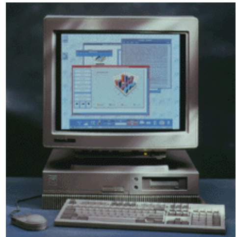
Automatic Satellite Acquisition & Processing (ASAP) interface permits sector definition, storage path and fiber/optic network routing.
